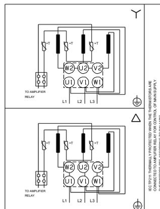
IEC 3111 THERMAL PROTECTED MOTOR THE THERMAL PROTECTORS ARE CONNECTED TO AMPLIFIER RELAY FOR CONTROL OF MOTOR SAFETY. THERMAL PTC ACCORDING TO DIN 4422.
