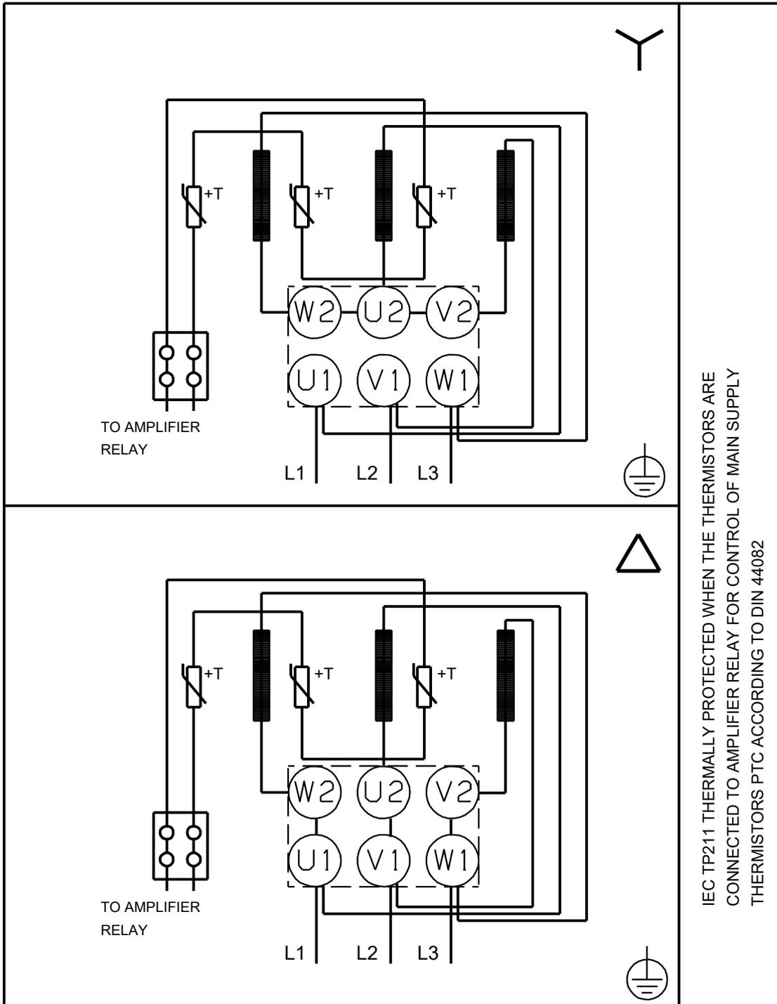
IEC TP211 THERMALLY PROTECTED WHEN THE THERMISTORS ARE CONNECTED TO AMPLIFIER RELAY FOR CONTROL OF MAIN SUPPLY THERMISTORS PTC ACCORDING TO DIN 44082
